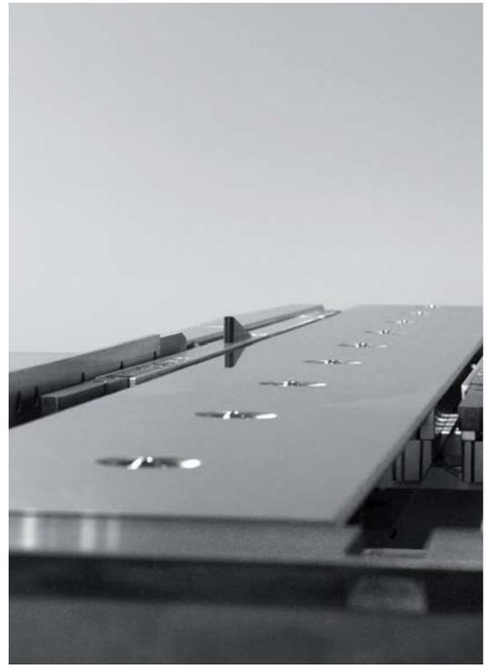
With the optional suction gauge all bends on one side can be done with one simple action by the operator.
