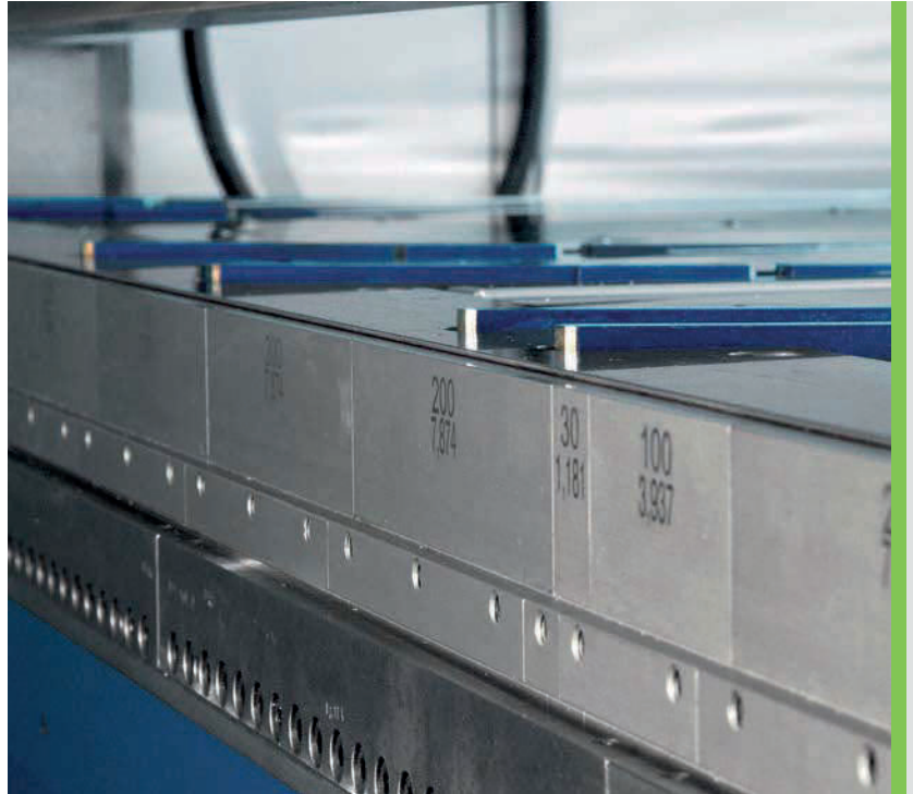
Segmented tools on the folding beam leave more space.
