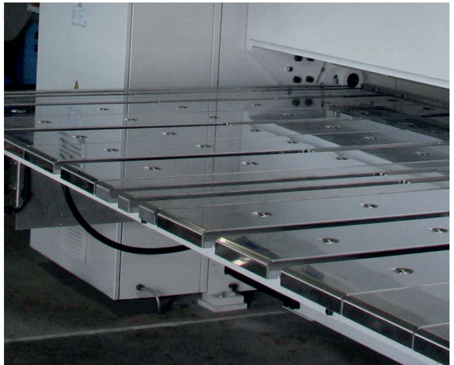
Gauge table, 1,600 mm, closed, with ball transfers
