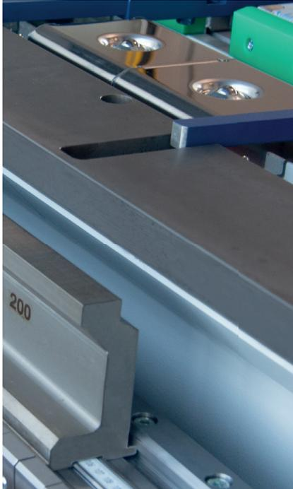
Bottom beam blade with finger grooves
