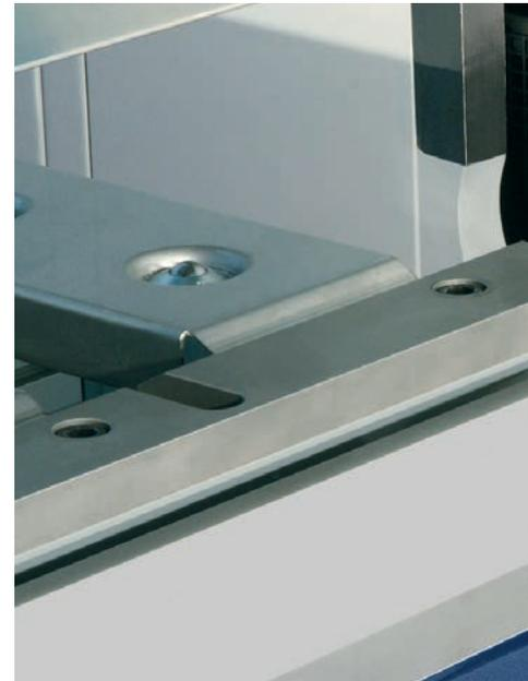
Motorized folding beam adjustment, 80 mm
