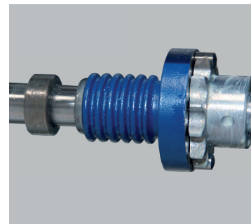
Standard: Coupling to adjust back roll or bottom roll
