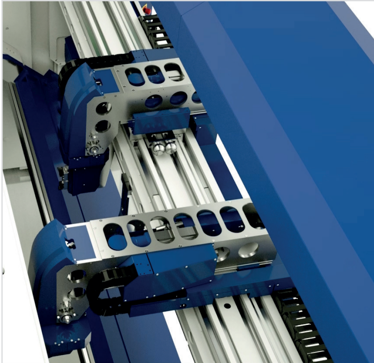
Two asynchronously movable tool changers each have a gripper unit.
