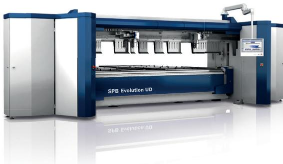
Just one click on our software control, and the fully automatic tool changer converts the clamping and folding beam for the next order in just a few seconds.
