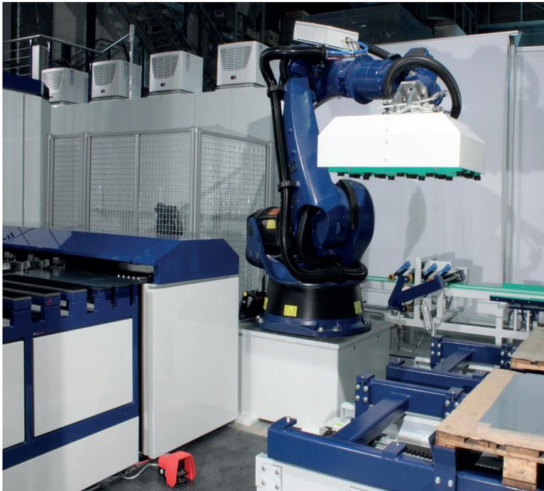
Kuka-Roboter in operation: The sheet gets picked up via suction units
