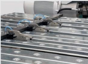
As optional equipment, the Schröder Group offers the so-called MAH21 motorized back gauge. With pneumatically controlled grippers it leaves nothing to be desired by the operator. The grippers can grip the sheet precisely and reliably. They are driven by recirculated ball screws.
