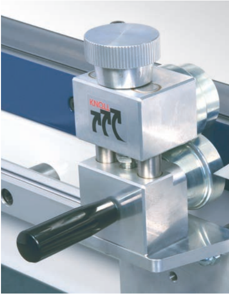
The profiling and flattening wheels are used to give the piece the required shape.
