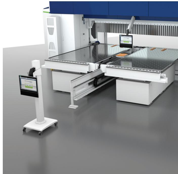
Additional operator terminal on the rear - free-standing column turnable and height-adjustable.
